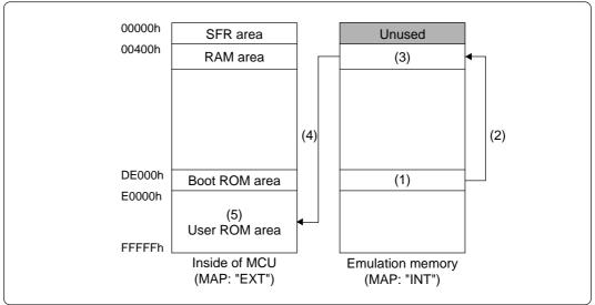
Figure 4.3 Memory map when debugging in boot mode
